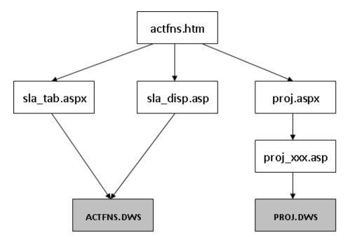
The diagram above illustrates the structure of the web application and the various files involved. The starting page, actfns.htm, simply provides a menu of choices which link to various .aspx web pages. These pages in turn are linked to one of the two workspaces via the src=""declaration"
