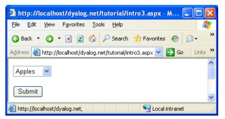
In this example, the page is processed by a POST back caused by pressing the Submit button. As it stands, changing the selection in the list object does not cause the text in the out object to be changed; you have to press the Submit button first.
